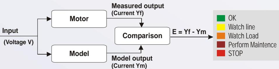
PA-01 detects both electrical and mechanical faults just by measuring three-phase voltage and current signals of motor. The relationship between input (voltage) and output (current) is very sensitive to mechanical changes in motor. Since such changes affect the calculated parameters, it is possible to detect mechanical faults in a very early stage.
